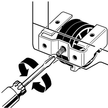
3. Depending on your model, to level your refrigerator you may either turn the screw clockwise to raise that side of the refrigerator or turn the screw counterclockwise to lower that side. Place a level on top of the refrigerator to check adjustments.
